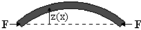
FIG. 4. When a force F is applied to the ends of a beam it remains horizontal until the force exceeds a critical value F_c .
